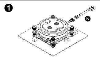
Install the Water Block on the mainboard properly, and connect the water block cable to the conversion cable.
