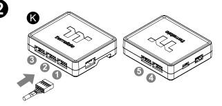
Connect the plug into the port in numerical order, start with plug one.
