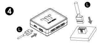
Connect the controller cable onto the mainboard (USB 2.0 9 pin) and controller.
