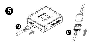
Connect the power cable to the 4pin Molex connecter and controller.
